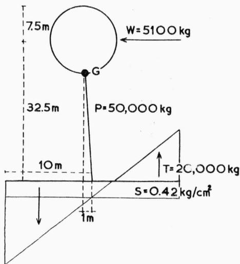
Fig. 2. — Diagram of the tension force ( $T$ ) exerted upon a horizontal root of a large tree of *Entandrophragma angolense*;  $P$  — weight of the biomass of the tree,  $S$  — force weighing down 4 main horizontal roots,  $G$  — centre of gravity,  $W$  — force exerted by wind speed of 80 km per hour.
